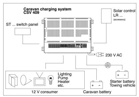
Fig. 1 Onboard power supply system
